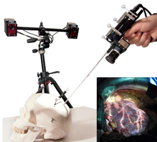
Actual prototype and projector-based visualization of vessels onto the human head and liver as an example of a deformable organ.
