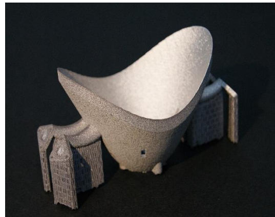
Figure 21: Additive manufactured reflector of an automotive headlight
